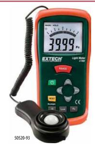
What's included: Light sensor with protective cover, protective holster, and 9 V battery.
